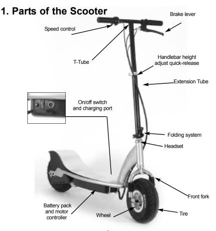
NOTE: Do not activate the speed control on the t-tube unless you are on the scooter and in a safe, outdoor environment suitable for riding. The E100 must be going 3 mph before motor will start.
